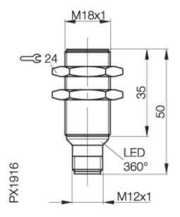
**Inductive Sensors** BES M18MF-USC70B-S04K M18x1 x 50 normally-open Sn=7mm shielded
